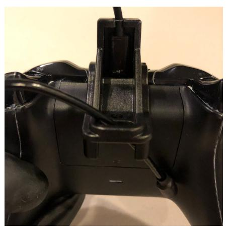
Align the bracket and the cable so it surrounds the top of the controller. Make sure to insert the USB cable into the round slot located at the top of the bracket.
