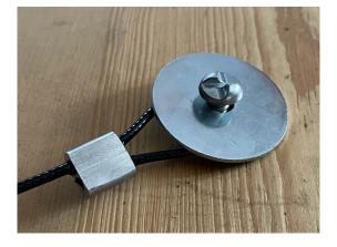
Pre-drill the hole that you will be using to attach the security cable using the provided security screw and washer. Insert the security screw into the hole of the washer and place this on top of the eyelet on the security cable and use the provided screwdriver bit to secure the cable to the surface.
