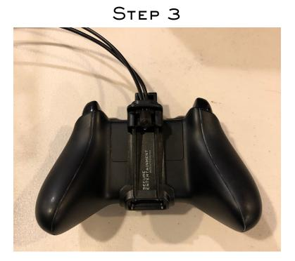
Next, take the bottom part of the bracket and place it onto the controller from the bottom making sure to align the security cable into the slot in the bracket.
