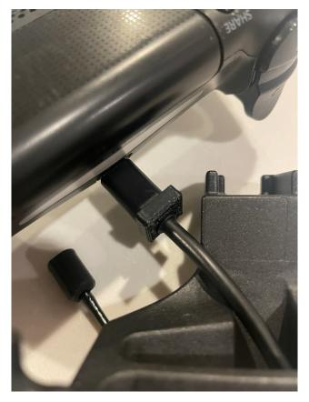
Align the bracket and the cable so it surrounds the top of the controller. Make sure to insert the USB cable into the round slot located at the top of the bracket. Clip on the plastic shim that was included in the packaging around the USB cable head.
