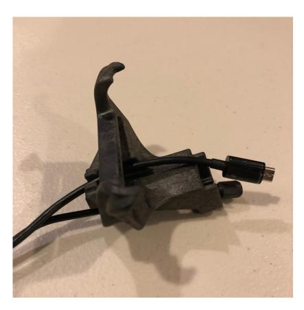
Grab bracket part shown above and feed USB plug that connects to the controller through opening that lines up with the USB slot on the controller. Plug in the USB cable to the controller. Insert the barrel end of the security cable into the rectangular opening on the bottom of the bracket.
