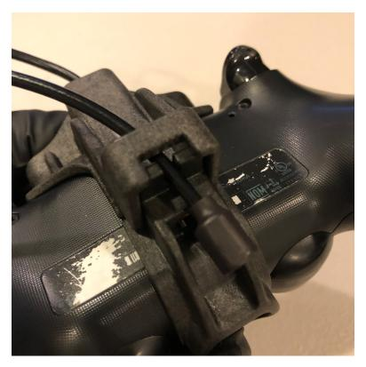
Next, take the bottom part of the bracket and place it onto the controller from the bottom making sure to align the security cable into the slot in the bracket.
