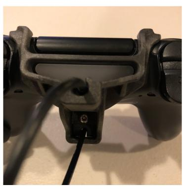
From the top of the bracket. Insert the security screw and tighten using the screwdriver bit provided
