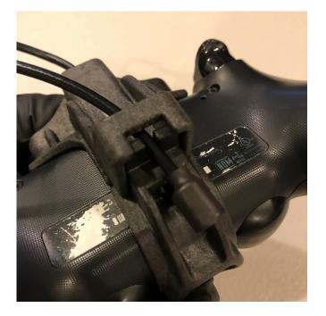
Next, take the bottom part of the bracket and place it onto the controller from the bottom making sure to align the security cable into the slot in the bracket.
