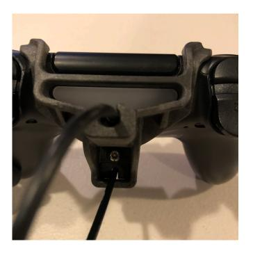
From the top of the bracket. Insert the security screw and tighten using the screwdriver bit provided (screwdriver not included)
