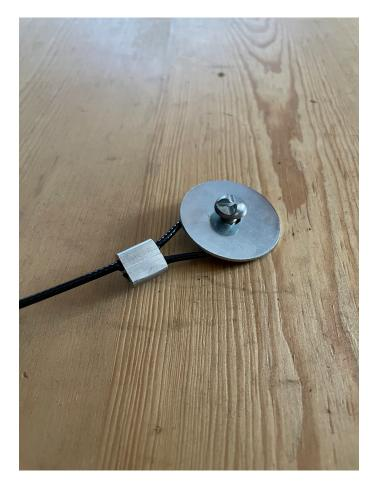
Pre-drill the hole that you will be using to attach the security cable using the provided security screw and washer. Insert the security screw into the hole of the washer and place this on top of the eyelet on the security cable and use a flathead screwdriver to screw in the screw into the secure surface. Be aware that these screws can only be tightened. If you wish to remove the cable from this surface at a later date, we suggest using a different screw of your choosing.
