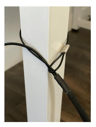
Optionally, you can wrap the security cable around a secure piece of furniture. Simply wrap the cable around the location you want to install and pass through the USB and the other end of the security cable through the loop.
