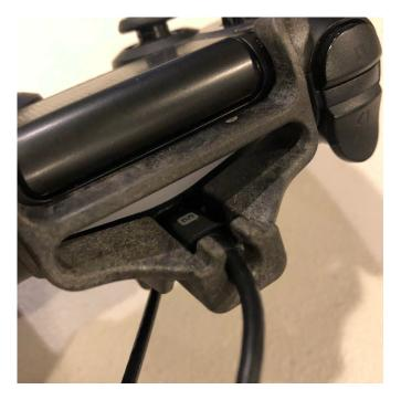
Align the bracket and the cable so it surrounds the top of the controller. Make sure to insert the cable into the round slot located at the top of the bracket.
